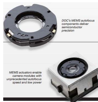
Chart 74. Auto-focusing actuator using MEMS technology
