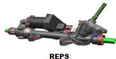
Figure 45: Nexteer REPS for ADAS Level 4
