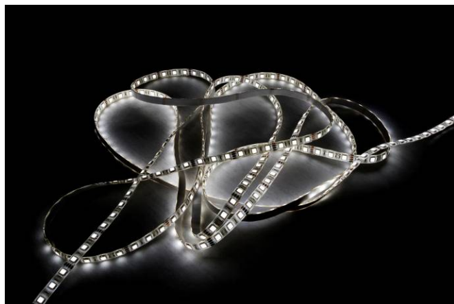
Figure 118: White LED strip used in TV backlighting
