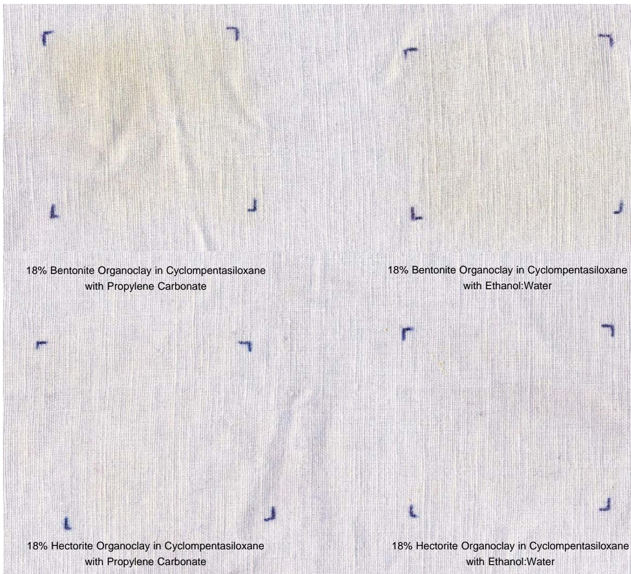
Figure 14. Stain intensity of hydrophobic organoclays in Cyclompentasiloxane following six (6) treatment cycles
