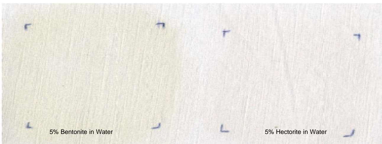
Figure 13. Stain intensity of aqueous dispersions of hydrophilic clays following six (6) treatment cycles
