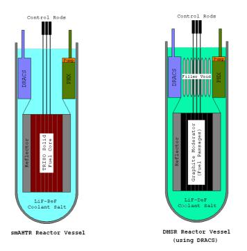
Figure 1 The ORNL SmAHTR.design on left and a simple DMSR counterpart on the right
