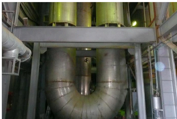
Exhibit 60: Akdala, U-shaped Ion Exchange Column
