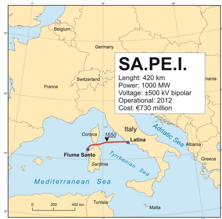
Fig. 40 – SA.PE.I. HVDC submarine power cable in Italy between Sardinia and the peninsula
