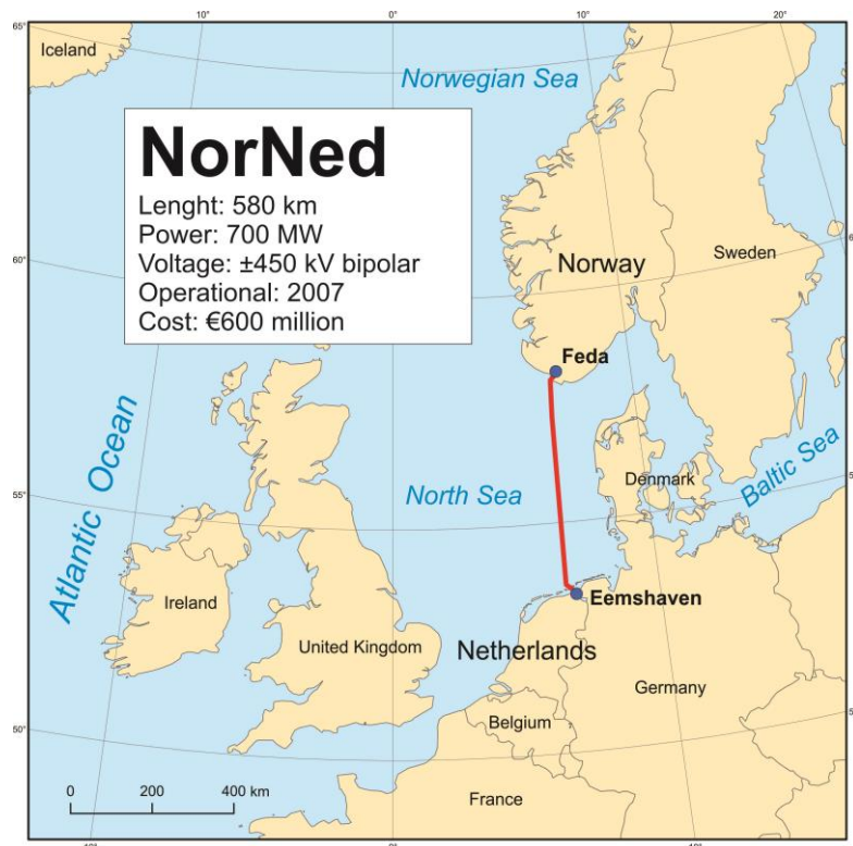
Fig. 39 – NorNed HVDC submarine power cable between Norway and The Netherlands
