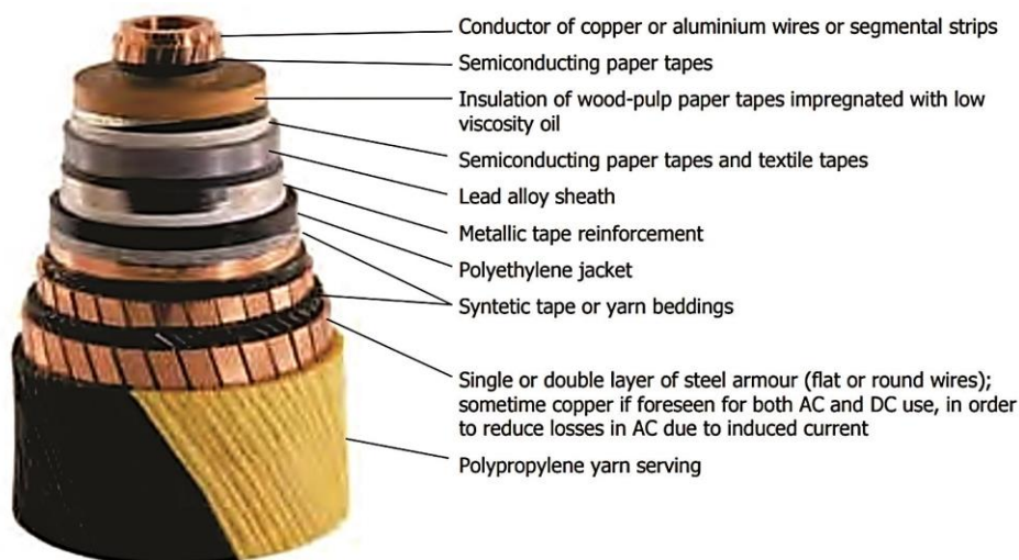
Fig. 25 – The structure of a self-contained fluid-filled cable (Zaccone, 2009)
