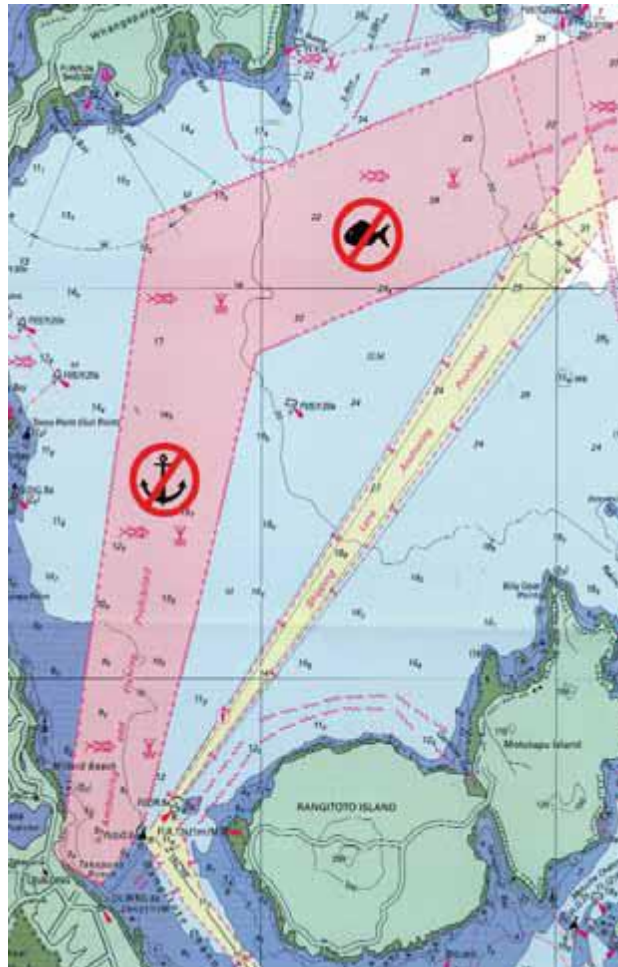
Fig. 34 – Cable Protection Zone in New Zealand (Carter et al., 2009)
