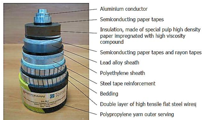
Fig. 42 – The structure of the deep water segment of the SA.PE.I power cable (Rendina et al., 2012)
