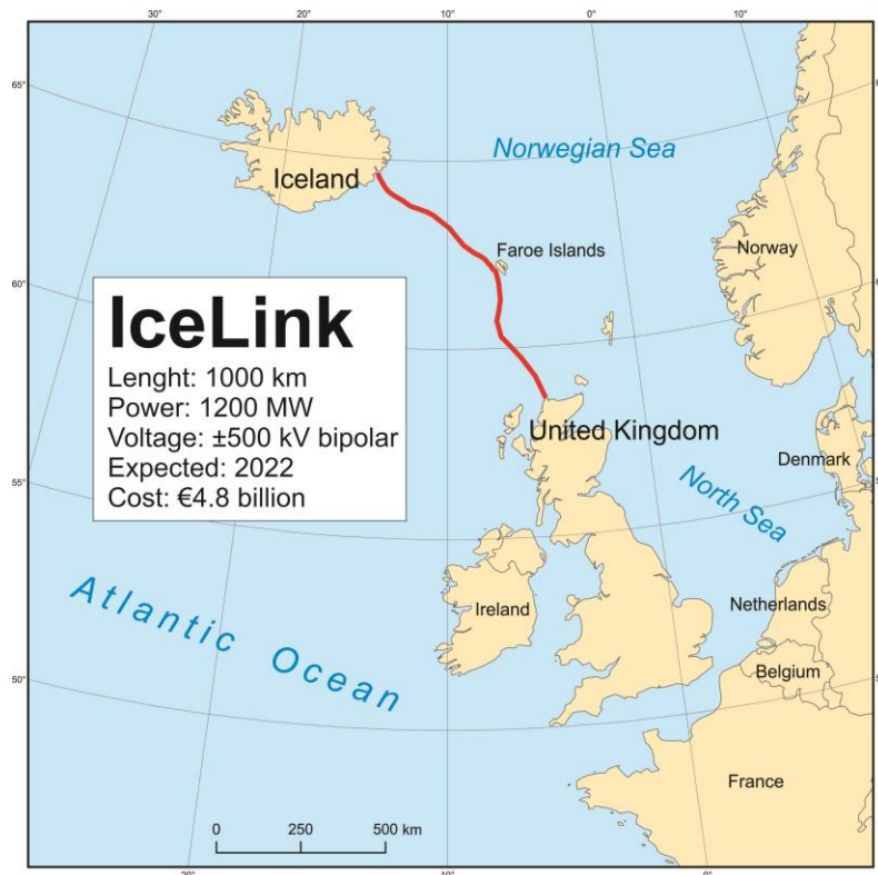
Fig. 48 – Future IceLink HVDC submarine power cable route between Iceland and United Kingdom
