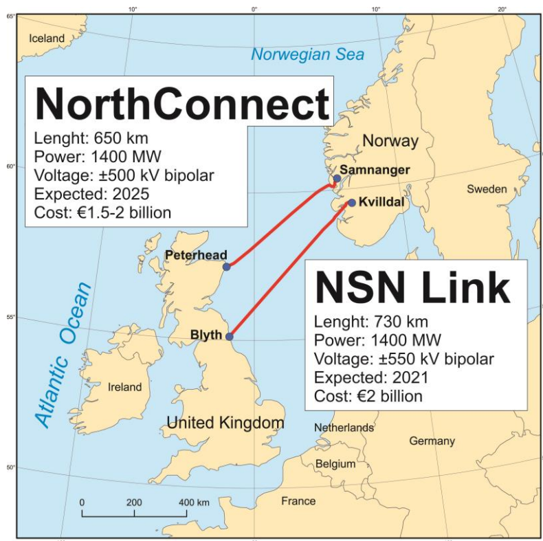
Fig. 46 – Future NSN Link and NorthConnect HVDC submarine power cable routes between Norway and United Kingdom
