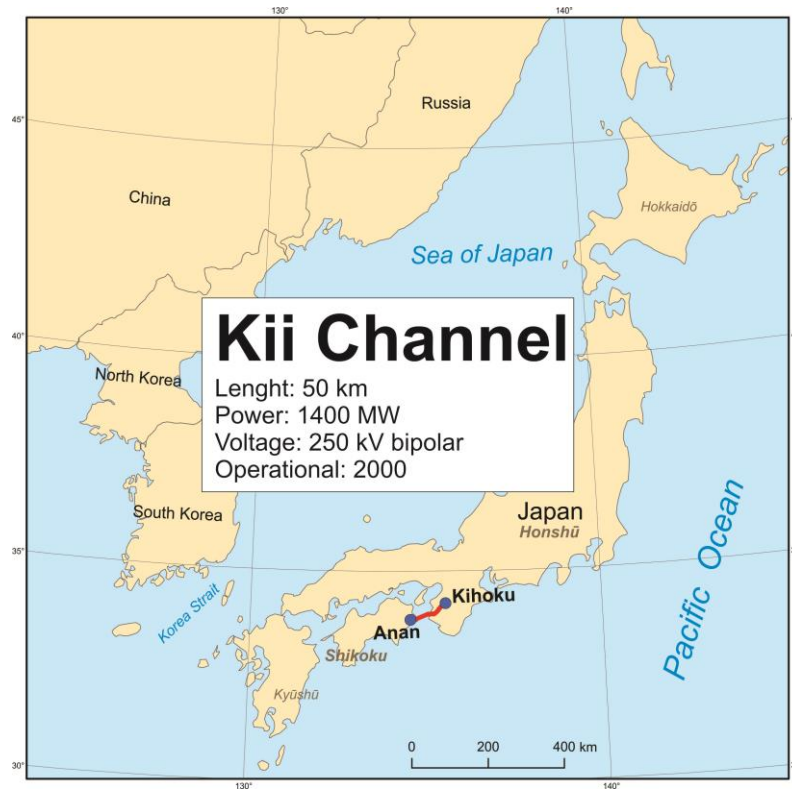
Fig. 45 – Kii Channel HVDC submarine power cable in Japan
