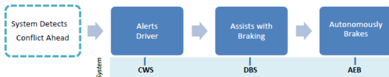
Figure 34: Collision avoidance system overview
