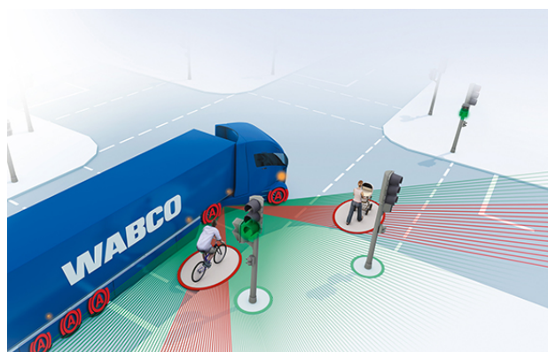
Figure 46: OnCity system uses LiDAR technology to detect obstacles when turning
