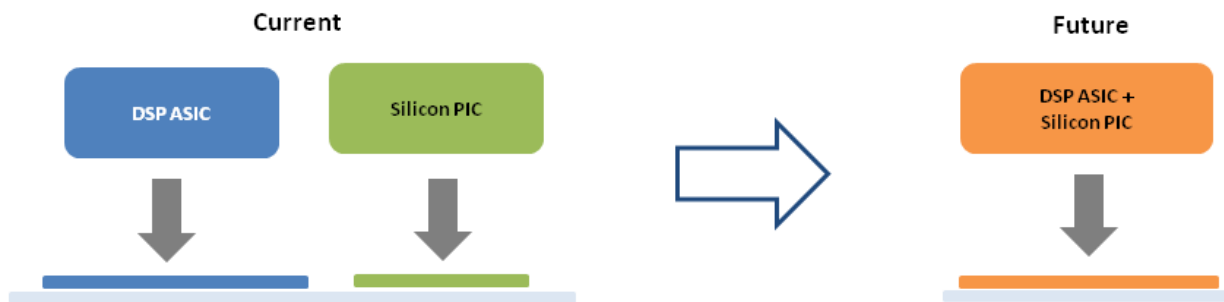
Figure 43: DB View of the Future of Optical: Consolidated DSP and Silicon PIC
