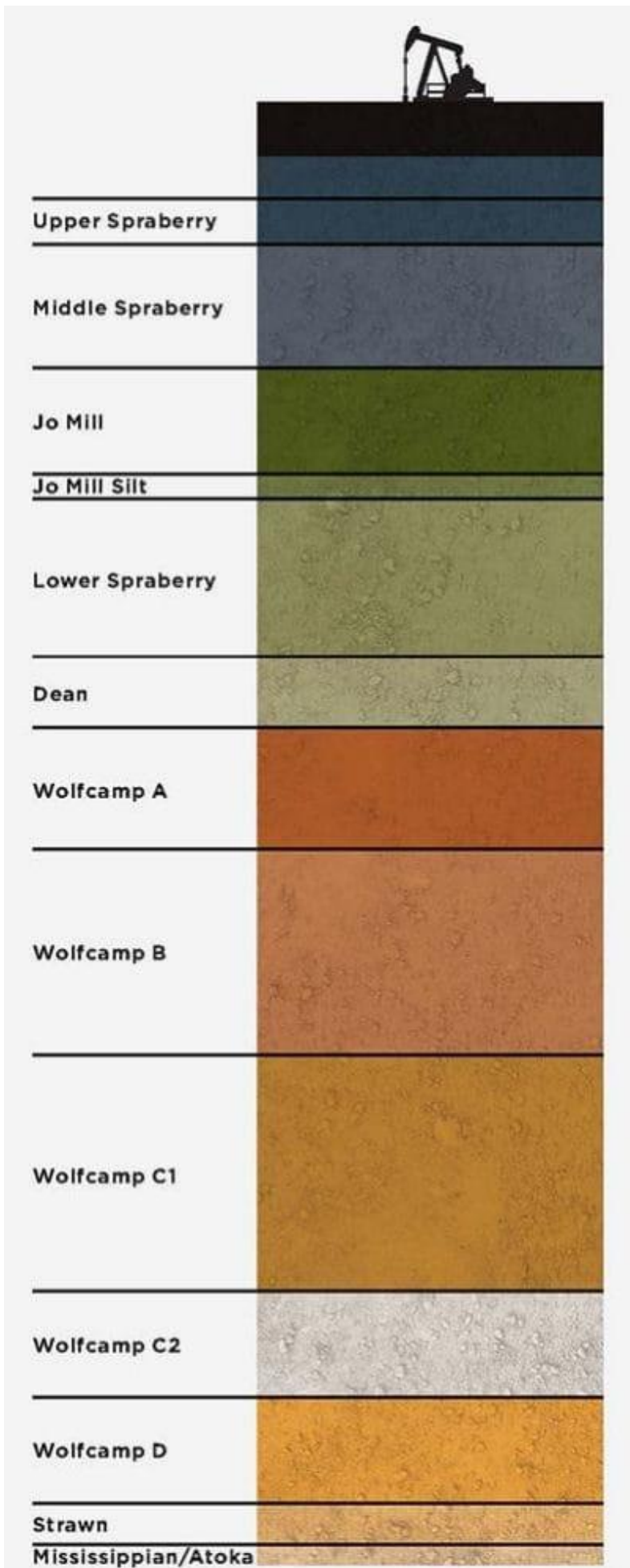
The Permian basin has many layers which boost extraction CREDIT: PIONEER NATURAL RESOURCES COMPANY
