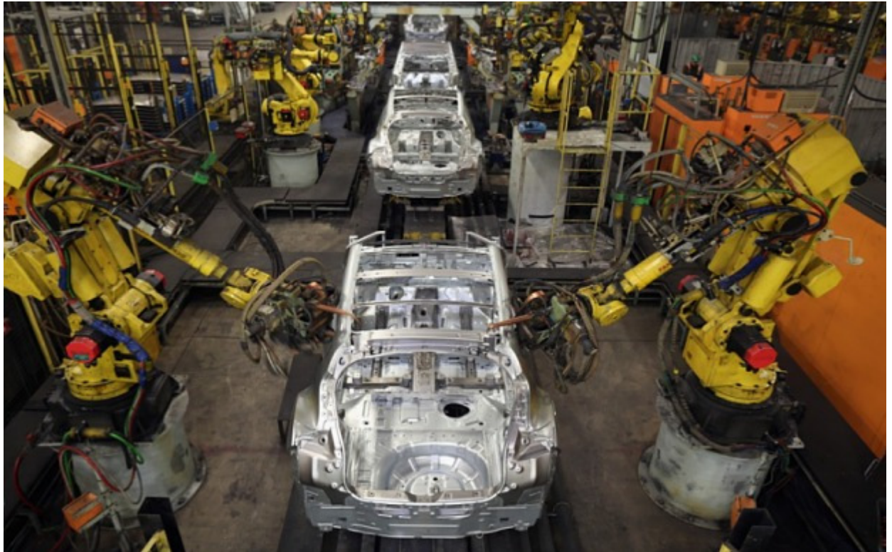
Robotic arms assemble and weld the body shell of a Nissan car in Sunderland Photo: Getty
