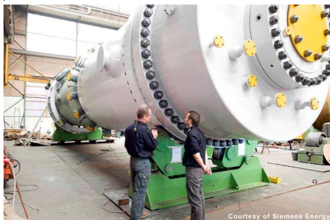
Figure 29: Coal gasifier (Shenhua CTL)
